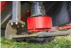
Direct drive from the gearbox to the first disc for efficient power transmission.
