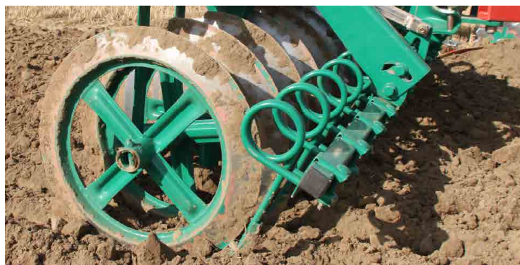
Single front harrow: 16 mm tines with rev. points or 20 mm tines with blade points
