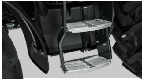
Left/Right 2 Steps Installed steps on both sides where the bottom level is adjustable to enable workers to easily get on and off anywhere. Installed plates help blow foreign residues from wheels.
