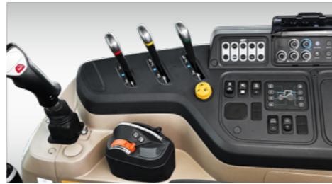
Grouping of Levers and Switches Levers and switches used to conduct similar tasks are grouped for better convenience.
