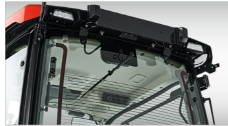
Front/Rear Wiper Enhanced the front wiper motor capacity while introducing user modes for improved performance, facilitating effortless visibility enhancement by effectively clearing away dirt and dust.
