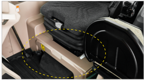
Bottom Seat Cover A beige injection cover has been applied to conceal exposed steel plates and bolts to complete a more refined environment.
