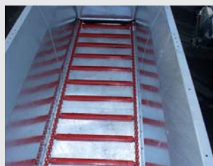
Straight body for easy cleaning 70 mm wide «U» slides
