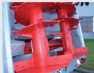
Beaters 1035 mm with 52 reversible cutters Oversized gearbox.
