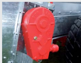
Oversized gearbox 10000 N.m with hydraulic motor 160 cm 3
