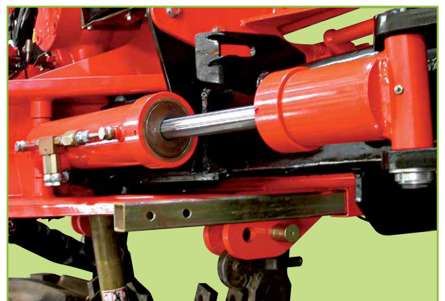
Erpici pieghevoli: Martinetti idraulici flottanti Klappbare Eggen: Schwimmend gelagerte Windenkolben Folding rotary harrow: floating hydraulic cylinder Herse repliables: verin flottant hydraulique
