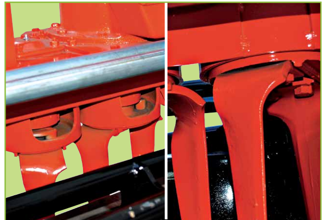
Protezione antisasso EPI Steinschutz für EPI Anti-stone protection EPI Protection anti-pierres EPI
