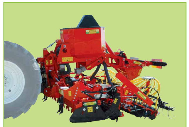
Combinata seminatrice pneumatica pieghevole: combisem sc-pne Klapp kombinierte pneumatische getreidesämaschine für kreiselegge Folding combined pneumatic grain seed drill for power harrow Association herse rotative-semoir pneumatique repliable
